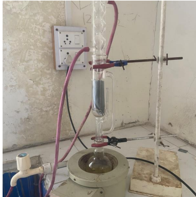
Fig.04: Extraction of Giloy by Soxhlet Apparatus
